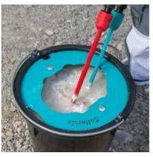
Place the dirty mixing paddle between the brushes, make the mixer rotate slowly until it is completely immersed. In order to guarantee that the mixer is cleaned properly, hold it in a slightly inclined position while it is rotating.
